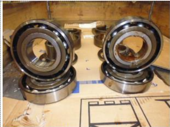
High stage, thrust bearing normal wear.
