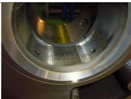
High stage, side bearing normal wear. Female side
