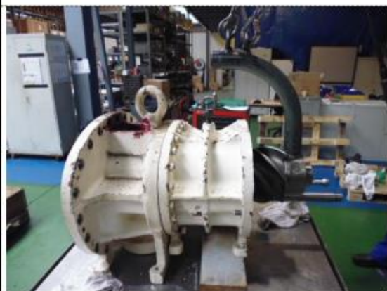
High stage, rotor assemblies. End clearance adjustment. Male side 0,07mm Female side 0,07mm (Specified range 0.05~0.07)
