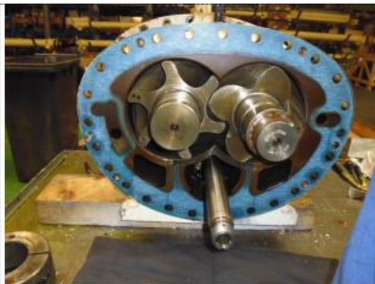
High stage, rotor disassembled.
