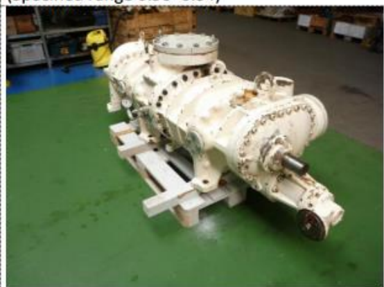
Compressor leak check. 20BarG.
