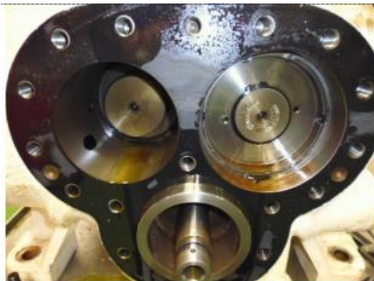
Balance piston cover disassembled.
