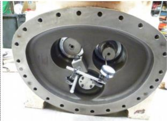
Low stage, end clearance adjustment. Male side 0,54mm Female side 0,54mm (Specified range 0.50~0.54)
