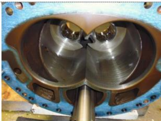
Inside rotor casing.
